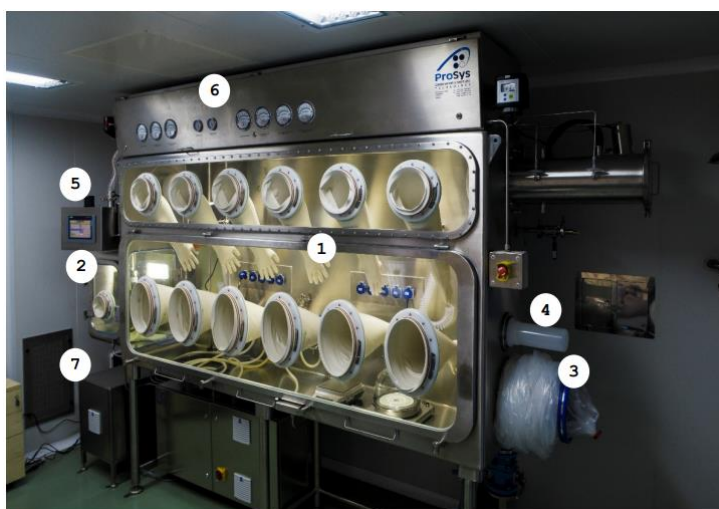
1: Main room, 2: Airlock room, 3: Continuous line, 4: RTP, 5: HMI, 6: LOP, 7: Fan
