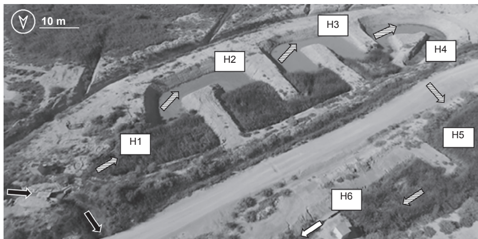
Fig. 1. CW design. Photograph of the surface flow CW with emergent macrophytes. The sampling points are depicted with white squares (H1 to H6), and the water flow within the CW with striped arrows. Non-treated water flow discharging to the Lerma gully is depicted with black arrows, and that of treated water with a white arrow.
