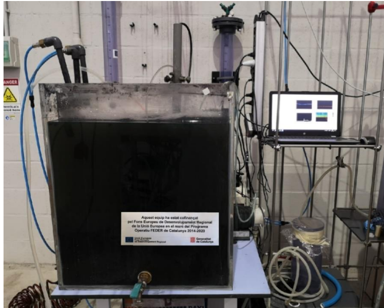
Figure III-6 Pilot plant of hybrid MBBR-MBR system
