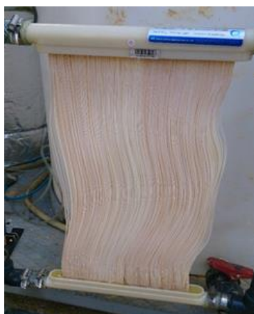
Figure III-7 MOTIMO BT01 hollow fiber flat plat membrane
