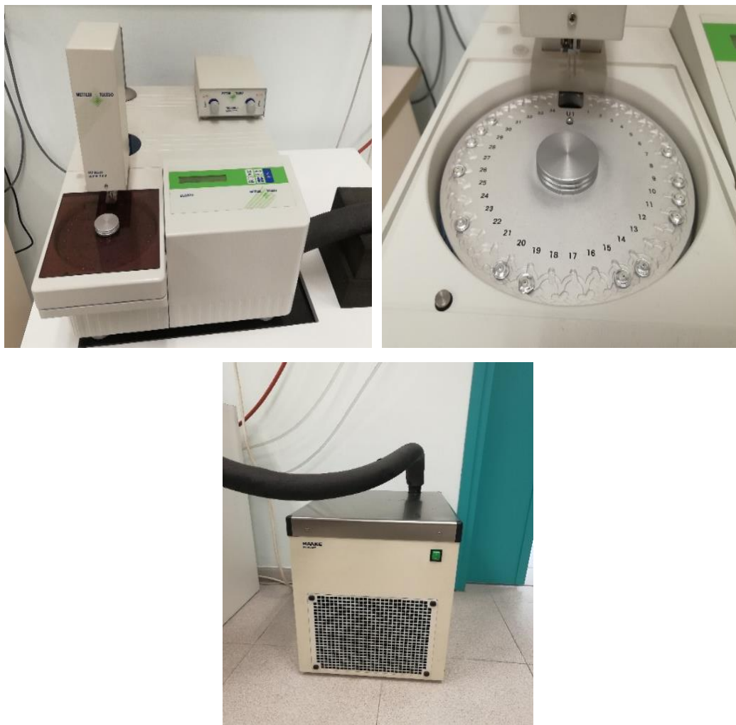
Figure 2.2. Top left, DSC machine; top right, the sample handler of DSC machine; bottom, intracooler.
