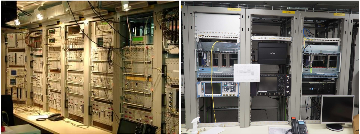
Fig. 6.3. Image of the SPS 200 MHz LLRF system in the Faraday cage: the pre-LIU SPS upgrade configuration (2018) (left), and the new configuration after the LIU SPS upgrade (right).
