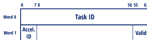
Figure 2.4: Format of elements in the finished queue
