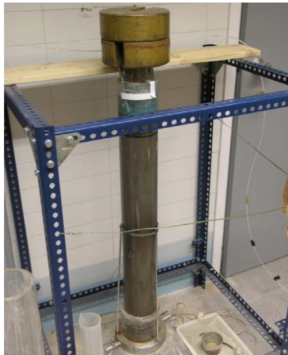
Figure F.3. Sedimentation test of hydraulic fill after the application of 45 kPa.
