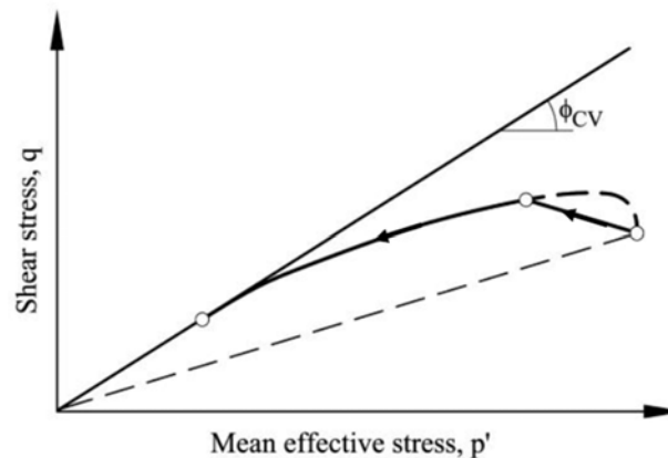
Figure 3.16. Drained unloading of lateral stress triggers flow liquefaction (Gens, 2019).
