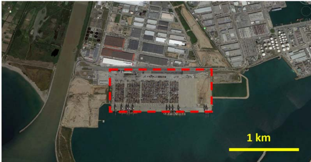
Figure 1.4. Satellite image showing Prat quay in 2020, originally designed with hydraulic fill, source Google Earth.
