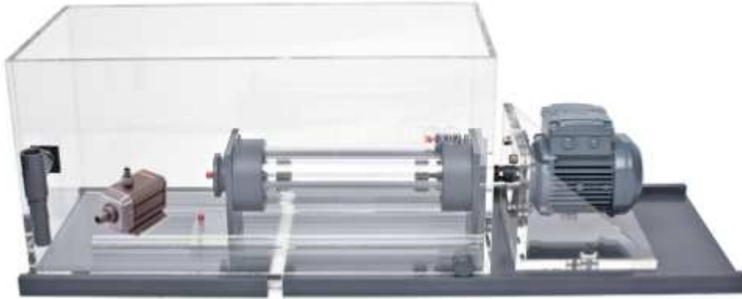
Figure 13. Respirometer (1.5 l) used for measurements of critical swimming capacity and metabolism. Image extracted from http://www.loligosystems.com .
