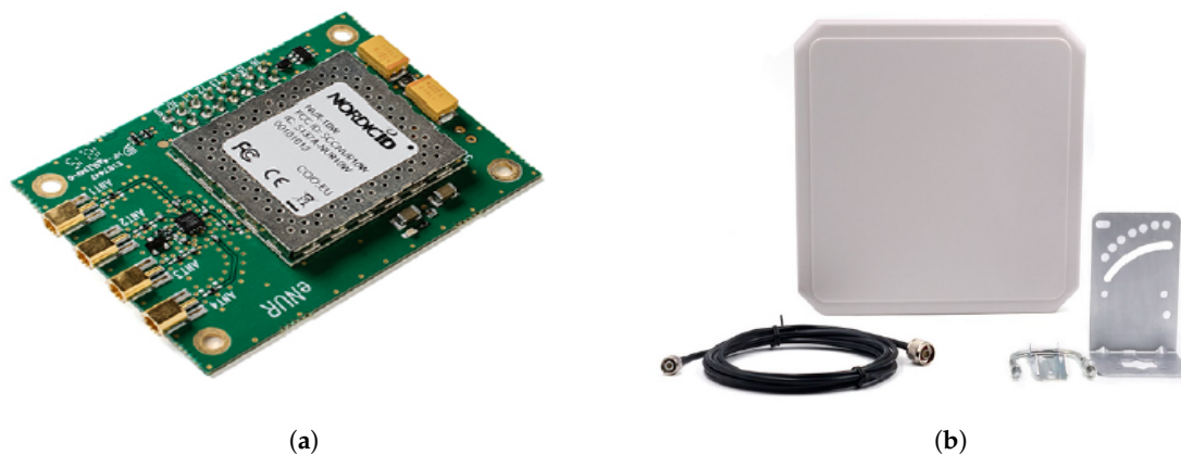
Figure 6. RFID Reader: (a) Nordic ID eNUR RFID reader and (b) antenna of the eNUR reader.
