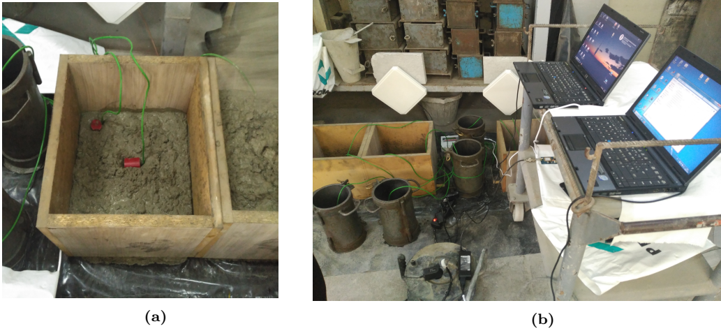
Figure 3.6: In-field measurement at PROMSA: (a) Location of the embedded RFID sensors and (b) layout of the whole measurement scenario.
