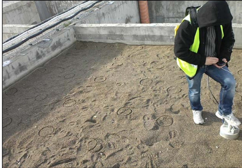
Figure 4. Collection of CO 2 soil-atmosphere fluxes on PISCO2 unit surface.
