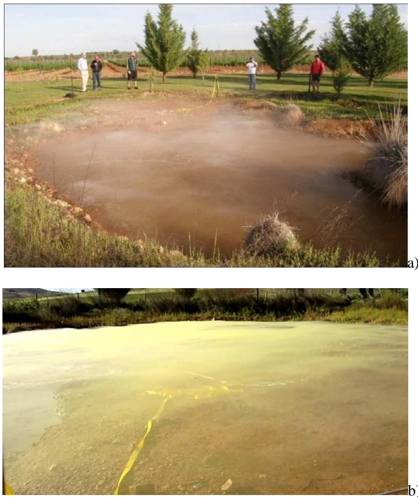
Figure 22. a) Formation of a CO 2 lake visible in the Cañada Real site, b) View of the Cañada Real site after lighting a smoke flare. The smoke (yellow) is not able to rise due to the denser blanket of the CO 2 -enriched air.
