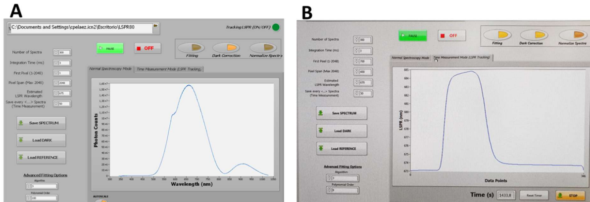
Figure 2.4 Screenshots of the homemade readout software showing in real-time the wavelength spectra (A) the spectroscopy mode (B) the time measurement mode for tracking of the position of the \lambda_{SPR} .
