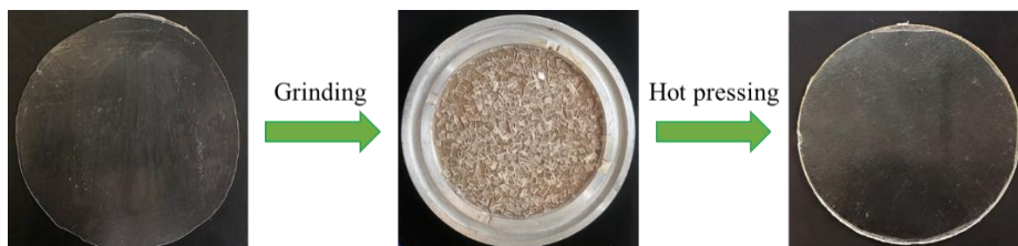
Figure VIII-8. Photographs of the original, grinded, and recycled sample prepared from stoichiometric PTU with a 0.1 % of BGDBU.
