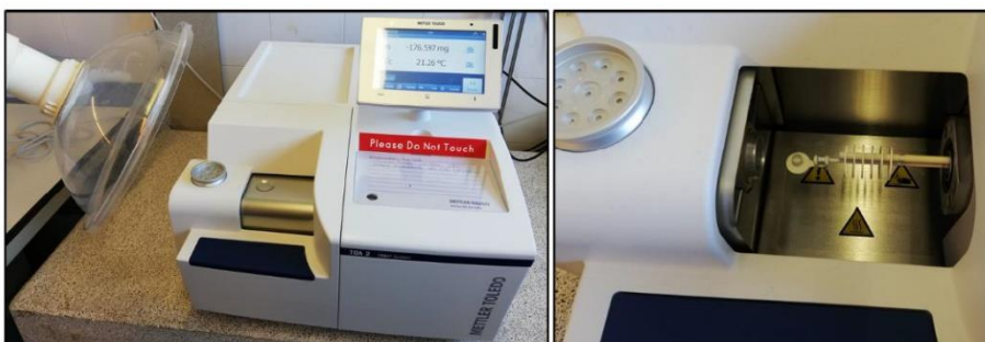
Figure II-3. Thermobalance Mettler TGA 2 (left) and a detailed image of the oven of the TGA (right).
