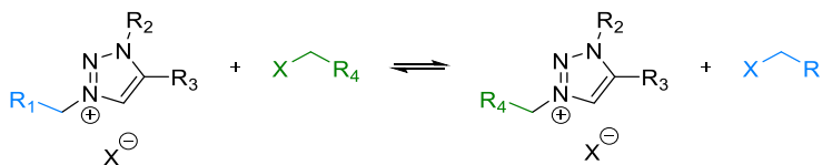
Figure I-22. Transalkylation exchange reaction of triazolium salts.
