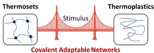
Figure I-5. Representation of the concept of covalent adaptable network.
