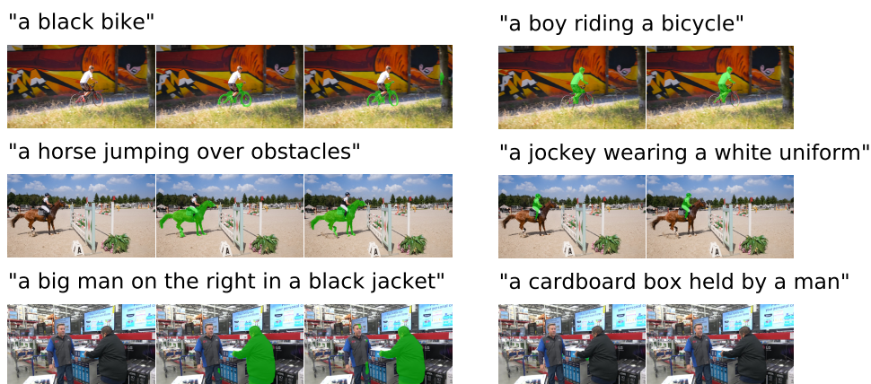
Figure 6.1: Video sequences for DAVIS 2017 with language queries and our results. The first column shows a reference frame, the second to third columns depict the masks produced by our model when given the language query shown on top. Finally, the fourth to fifth columns show the results for the language query shown on top of these columns, which refers to another object of the video sequence.
