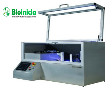
Figure II-10. Electrospinning equipment used. Fluidnatek® LE-10 from Bioinicia.
