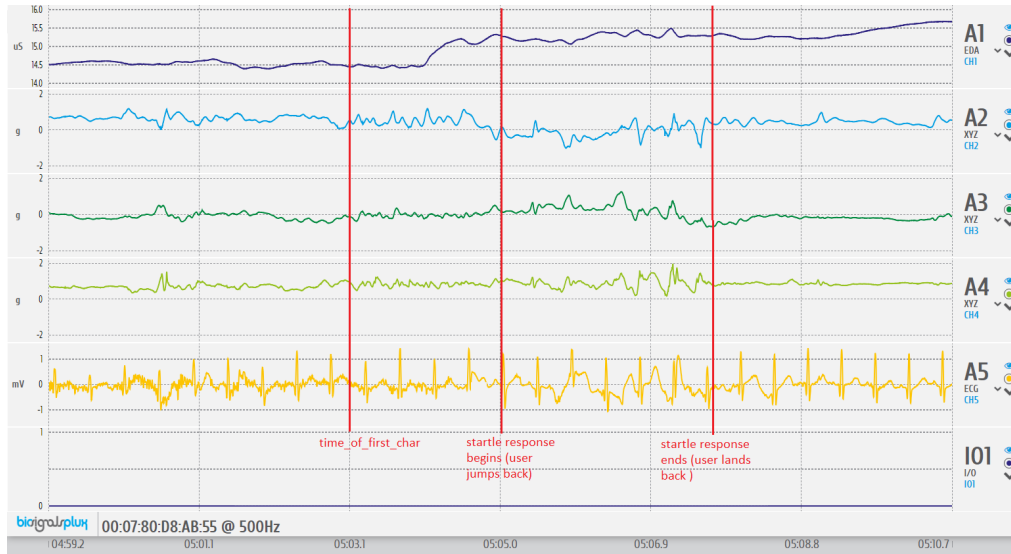
Figure 3.14: Opensignals [Osr, 2016], an open-source software to check the signal quality, view of raw psychophysiological signals in a 10 second window. Events are marked with red horizontal lines (time_of_first_char, startle response begins, startle response ends)
