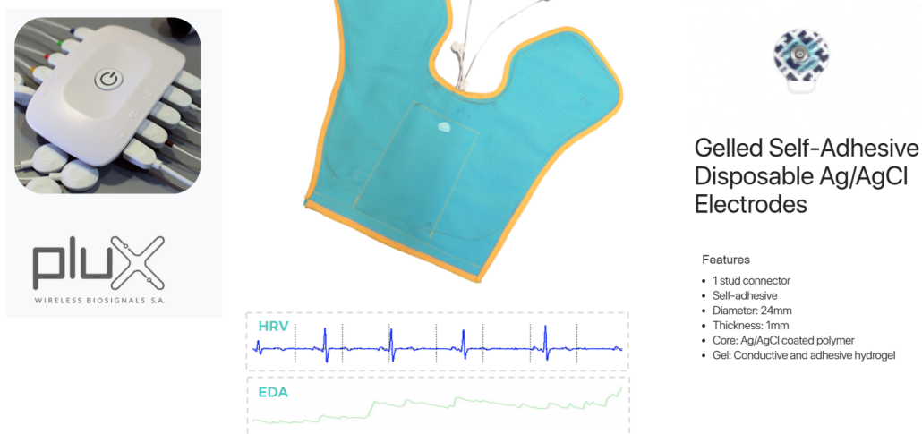
Figure 3.7: Views of biosignalplux research kit (left) / Superhero-collar wearable (middle) / gelled self-adhesive disposable Ag/AgCl electrode (right)
