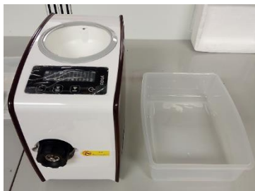
Figure 3.3 Screw pressing machine used to oil extraction from fresh and dry kernels pretreated by PEF.
