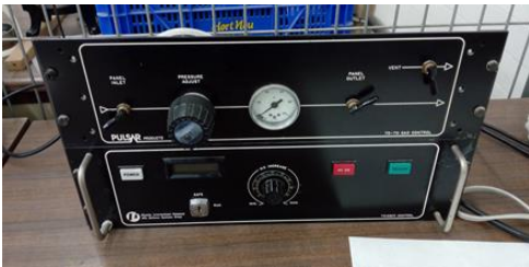
Figure 3.2 Pulse generator (PT-55, Pacific Atlantic Electronics Inc., USA) (a) and containers (b) to application of PEF.
