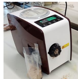
Figure 3.3 Screw pressing machine used to oil extraction from fresh and dry kernels pretreated by PEF.
