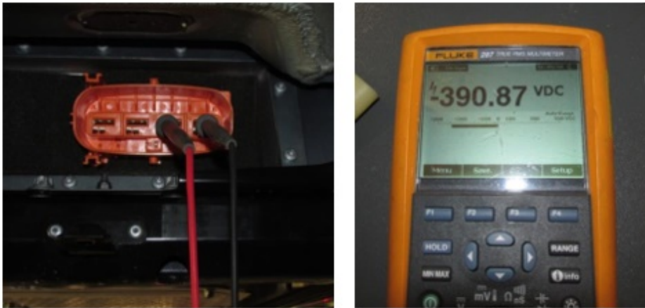
Figure 6.3: Battery voltage measurement before being disassembled
