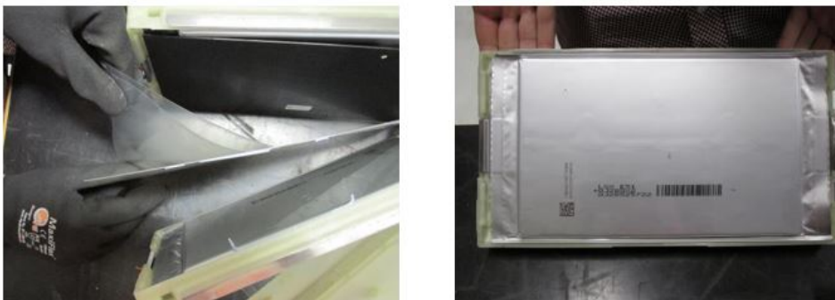
Figure 6.10: Right: Isolation between plates (three layers). Left: Cell on plate
