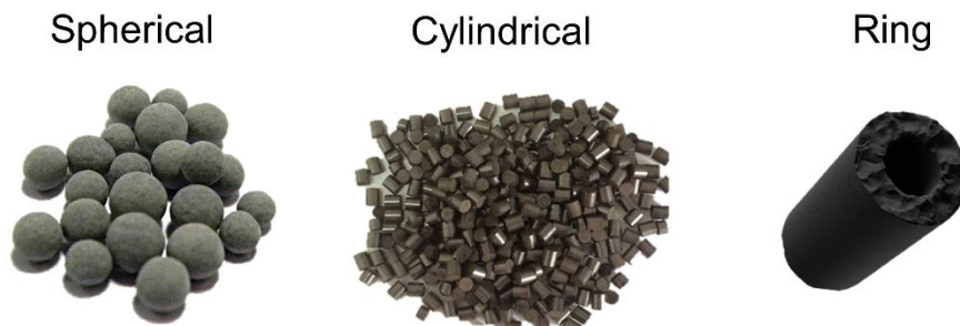
Figure 1.17. Commercial catalysts with different shapes for CO 2 methanation.
