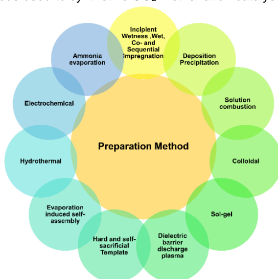
Figure 1.16. An overview of the preparation methods used to synthesize CO 2 methanation catalysts.
