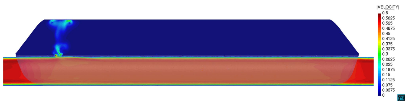
Fig. 7 Case A. Velocity cross section at t = 0.09 s. IF level set representation shadowed over the cross section
