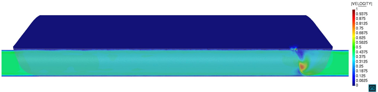
Fig. 8 Case B. Velocity cross section at t = 0.03 s. IF level set representation shadowed over the cross section
