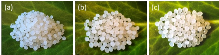
Figure 3.1. Photographs of the different grades of the PLA: (a) Futerro (b) 4032D and (c) 4043D used in the study
