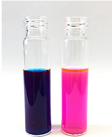
Figure 5-9. Crude extracts of A. platensis (left) and P. purpureum (right) grown in wastewater, showing abundance of phycocyanin and phycoerythrin, respectively.
