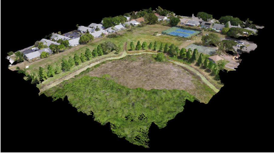
Figure 1.1 – Result obtained from a complete scene reconstruction pipeline. Reconstruction obtained using Open Drone Maps an open source photogrammetry toolkit to process aerial imagery into maps and 3D models. As can be seen, the global structure of the scene is very accurate after the combination of several computer vision techniques and multi-view geometry.
