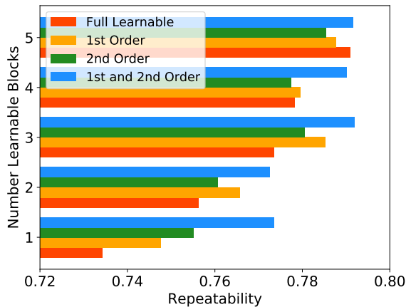
Figure 2.6 – Key.Net quantitative results for different learnable blocks. Repeatability results for different combinations of handcrafted filters and a number of learnable layers ( M = 8 filters each). A higher number of layers leads to better results. All repeatability scores are computed on synthetic validation set from ImageNet.
