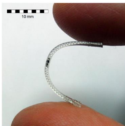
Figure 5 Dimensions and flexibility of a prototype of a non-addressable eAXON.
