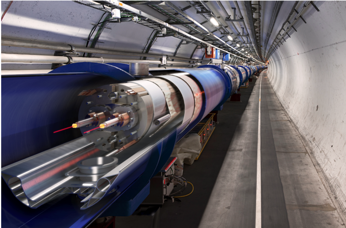
FIGURE 2.15: Cross section representation of the LHC MB in the tunnel, where the beam screens and the high radius of curvature of the 27 km long tunnel can be observed. Courtesy of CERN.
