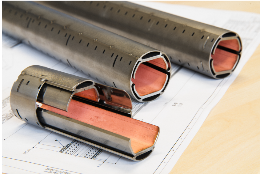
FIGURE 4.65: First prototypes of the FCC-hh BS. Manufactured by CERN.
