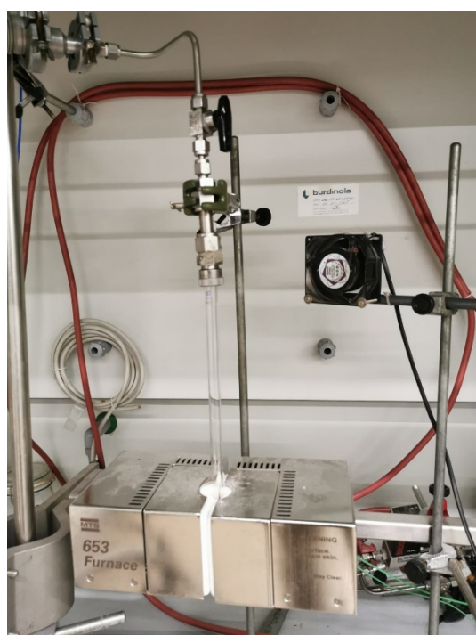
Figure 3.4. Picture of the home-made high-vacuum annealing set-up.
