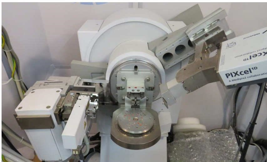
Figure 3.7. Picture of the Philips X'pert diffractometer from the UAB's X-ray diffraction facility.
