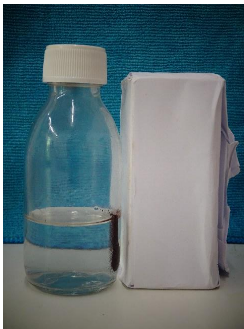
Fig. 4.6. Photo of magnetic separation.
