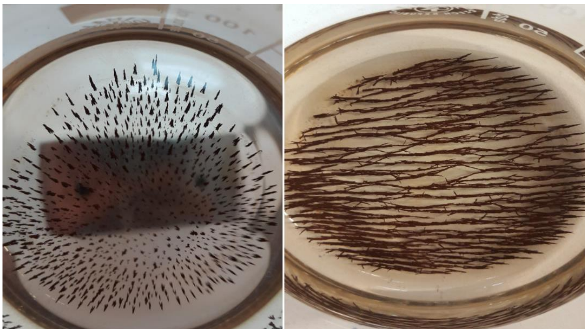
Fig. 4.3. Orientation of the \text{Ni}_{0.2}\text{Zn}_{0.2}\text{Fe}_{2.6}\text{O}_4 under a magnetic field.
