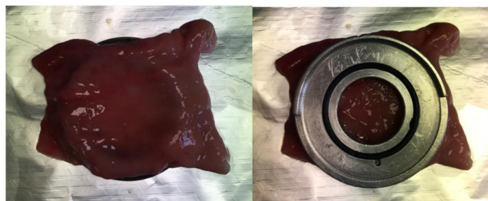
Figure 3. Piece of proximal small intestine of young female pigs ( Sus scrofa ) mounted on the metal ring of the Franz cells.
