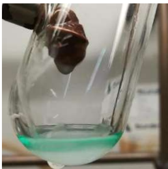
Figure S12. Digital image of the biphasic reaction mixture self-generated through the SET-LRP of \alpha PA in EtOH. The image was captured at 90 % conv. Reaction conditions: \alpha PA = 1 mL; EtOH = 0.5 mL; 4.5 cm hydrazine- activated Cu(0) wire; [\alpha\text{PA}]_0/[\text{EBiB}]_0/[\text{Me}_6\text{-TREN}]_0 = 25/1/0.1 .
