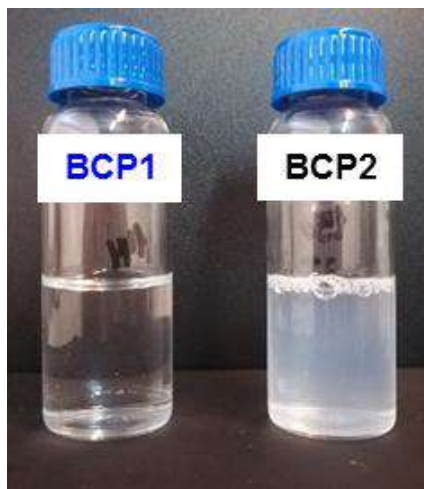
Figure S15. Digital images of images of self-assemblies from BCP1 ( 1 \text{ mg}\cdot\text{mL}^{-1} ) and BCP2 ( 0.5 \text{ mg}\cdot\text{mL}^{-1} ) in water.
