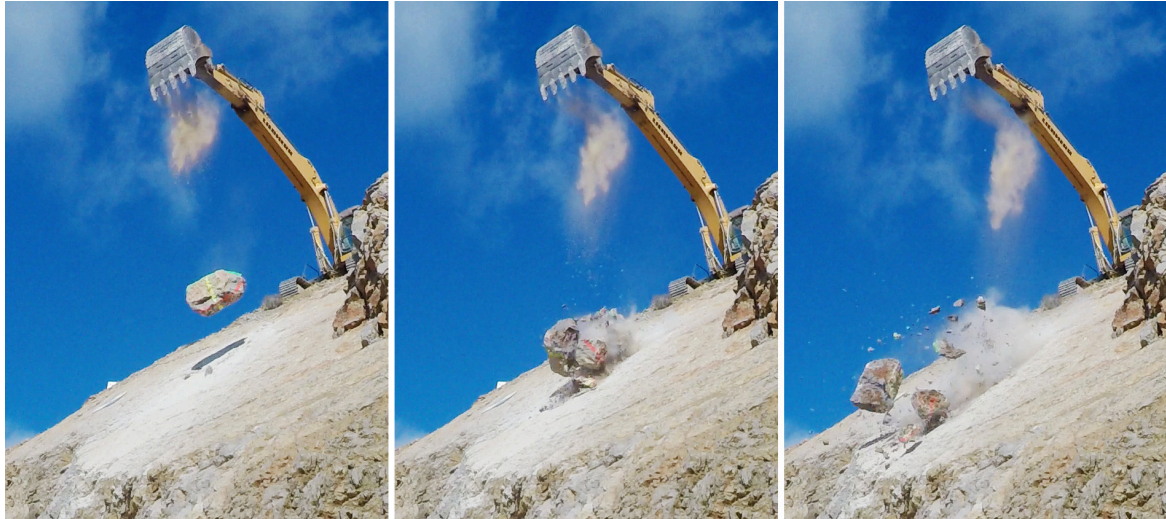
Figure 3.12: Example of the release of a block in test site #4. The time step between selected frames is 0.33 seconds. (Matas et al., 2020b)
