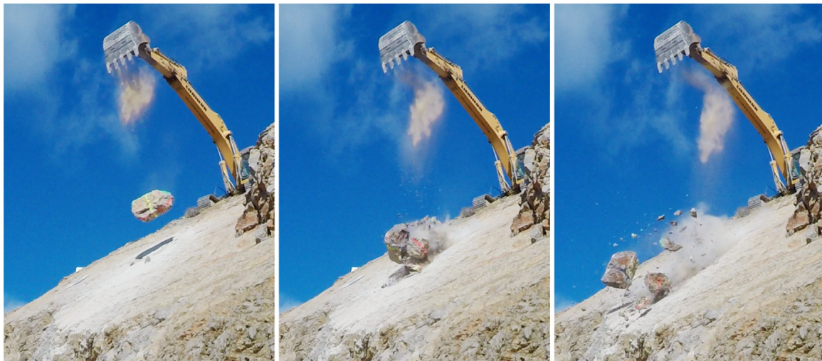
Figure 3. Example of the release of a block. The time step between selected frames is 0.33 s.
