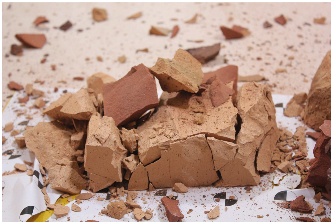
Figure 3.31: Detail of the bottom block of the release #60 (Figure 3.24) The cracking pattern is observed but the fragments in the middle remain in place like a puzzle
