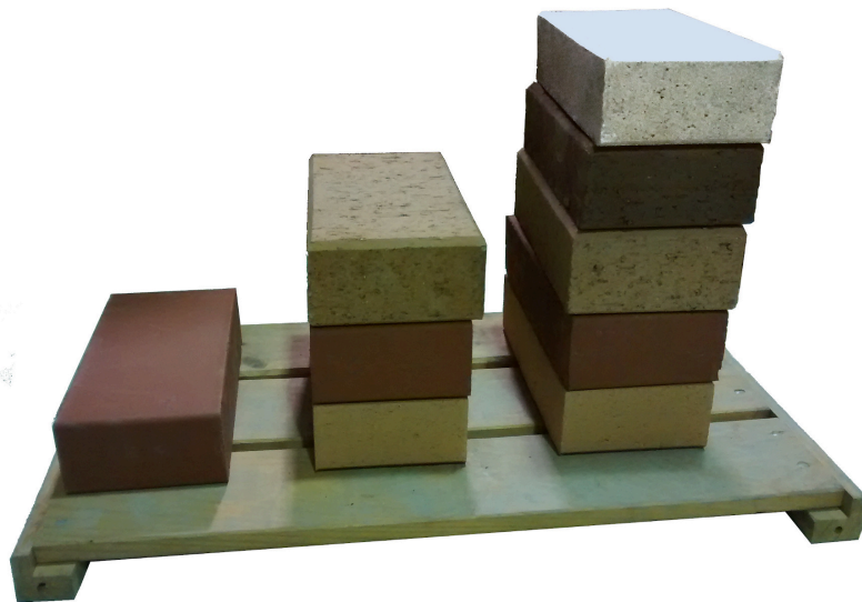
Figure 3.22: Possible stack distribution of bricks tested: single brick, three stacked and five stacked.
