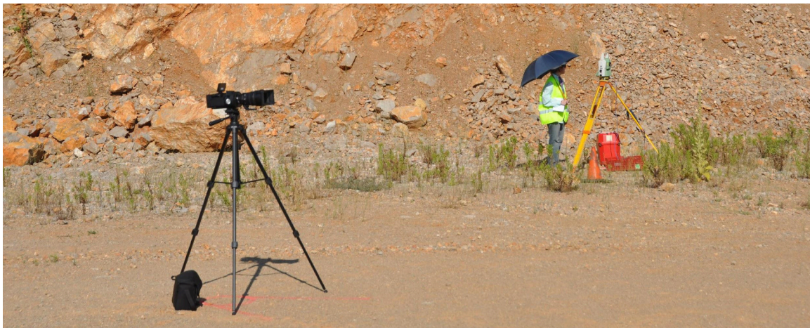
Figure 3.11: One of the high speed cameras used to record the tests and the total station used to georeference the ground control points placed on the scene.
