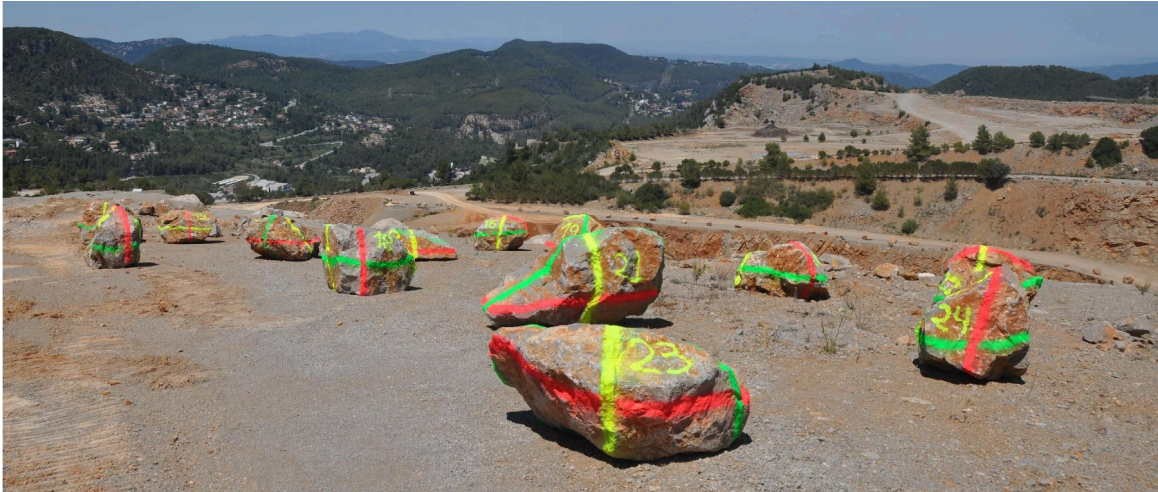
Figure 3.8: Blocks prepared for their release in testing site #1 being limestone the block lithology.
