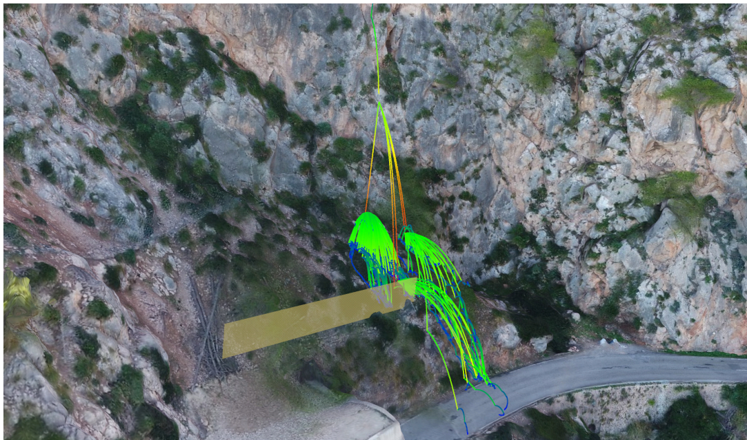
Figure 5.4: Reconstruction of the 10 \text{ m}^3 rockfall in Ma-10 Road in Mallorca. The runout calibration was done qualitatively considering the final position of the fragments reaching the road.
