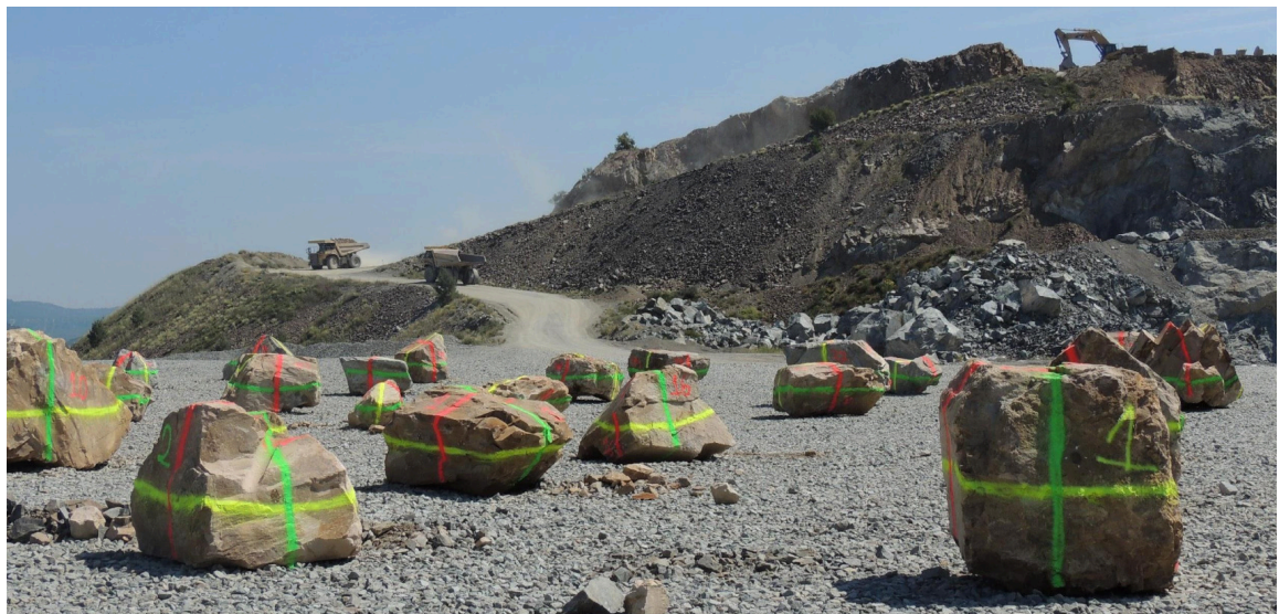
Figure 3.9: Blocks prepared for their release in testing site #3 being granite the block lithology.
