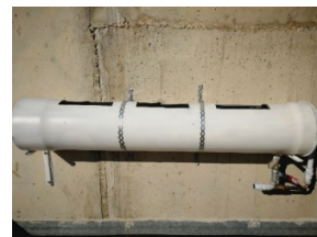
Figure 20 The WETWALL prototype – Fixation and allocation of the main structures (VF, HF and water reservoirs)
