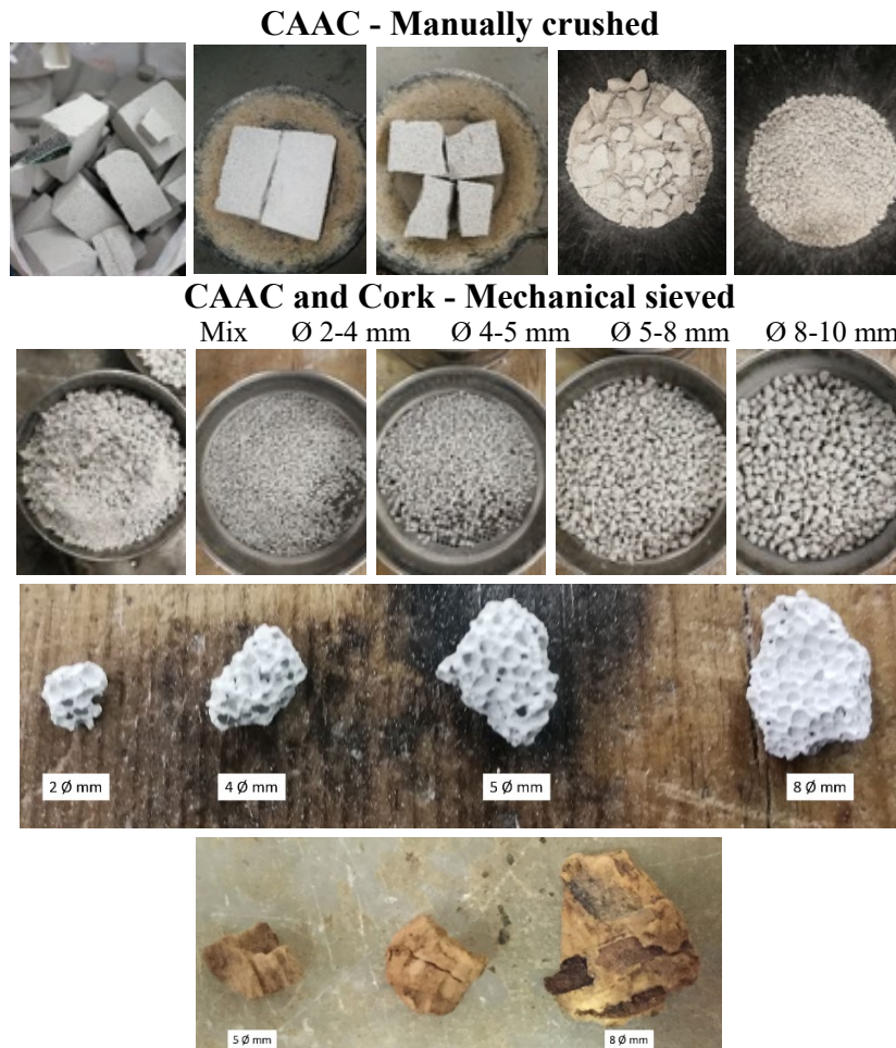
Figure 25 Main procedures for substrates preparation.
