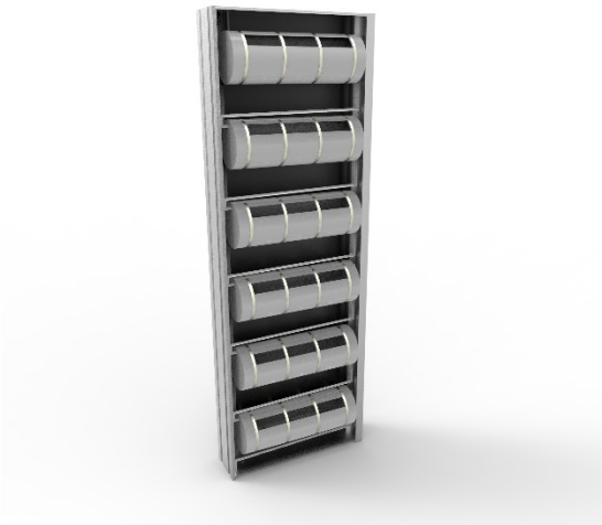
Figure 11 The WETWALL hybrid concept. Individual modules for each type of treatment (VF and HF)
