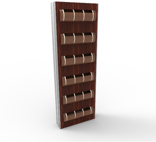
Figure 11 The WETWALL hybrid concept. Individual modules for each type of treatment (VF and HF)
