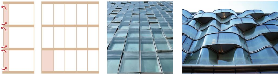
Figure 2.1. Box-Window DSF schematisation and examples.
