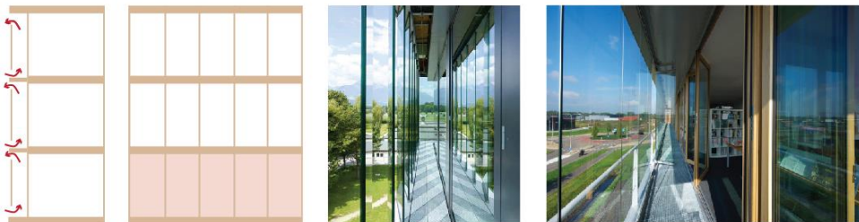
Figure 2.2. Corridor DSF schematisation and examples.
