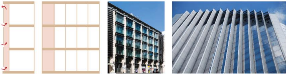
Figure 2.3. Shaft-Box DSF schematisation and examples.
