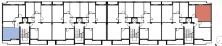
Figure 4.15. The localisation of the thermal zones selected for the winter (blue rectangle) and summer (red box) comfort.
