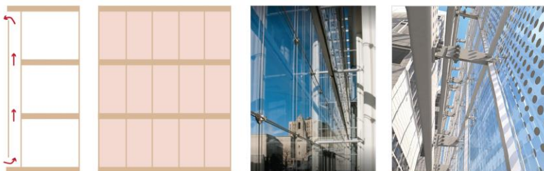
Figure 2.4. Multi-Storey DSF schematisation and examples.
