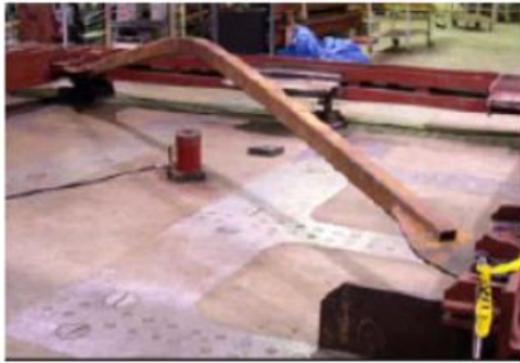
Traditional brace, buckled in compression
