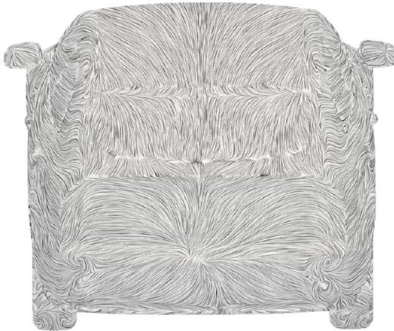
Figure 5.7: DrivAer. Streamlines for the average flow.
