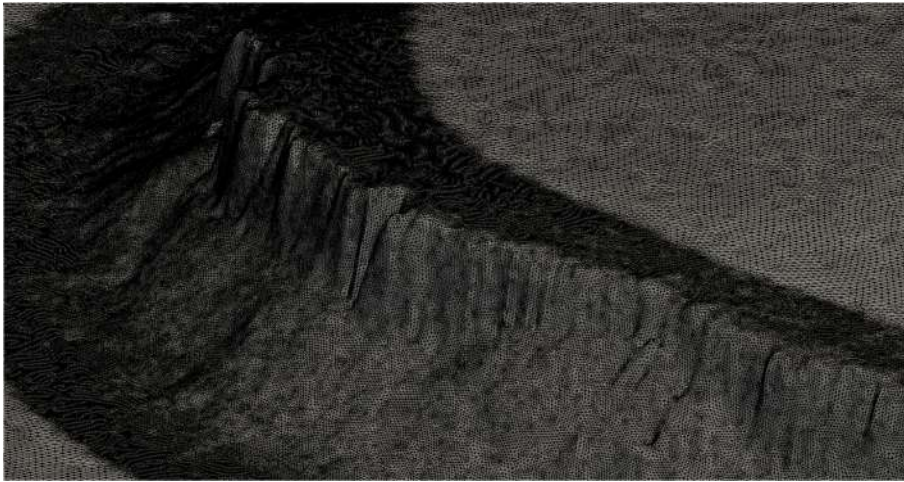
Figure 5.12: Detail of the Bolund hill surface mesh at the transition between the steeper vertical escarpment zone and the hill.
