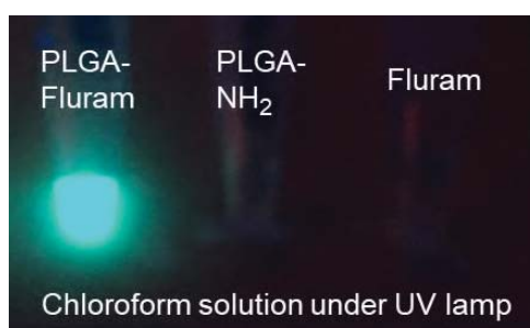
Figure 3-19. The corresponding polymer solutions under UV lamp. Only PLGA-Fluram shows green fluorescence.
