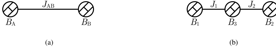
Figure D.1: Nodal scheme of (a) a two-node network coupled by an admittance inverter and (b) an equivalent three-nodes network.
