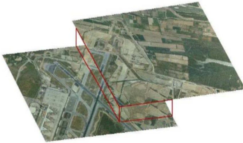
FIGURE 2.5: Overlapping area between two orthophotos to create an orthoimage
