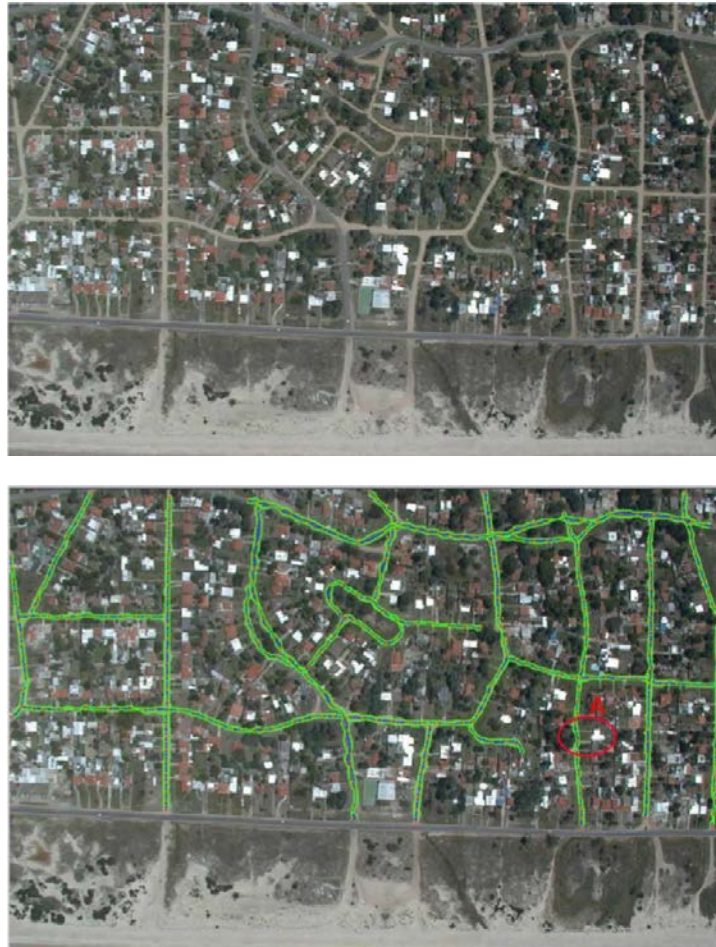
FIGURE 4.11: Original image and semi-automatic road extraction results obtained in the case of roads with light surrounding elements that could lead to the failure of the automatic process.
