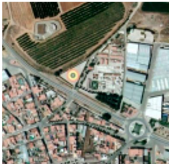
FIGURE 2.1: Image with 5m resolution on the terrain. Contrast lines and details are lost.
