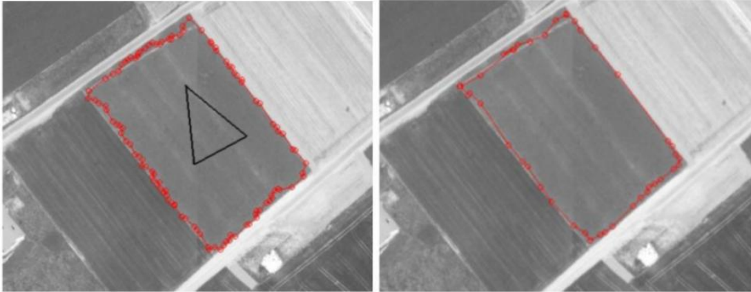
FIGURE 3.6: On the left, field extraction example with starting polygon (black) and extraction result without smoothing (red). On the right, extracted field after smoothing.
