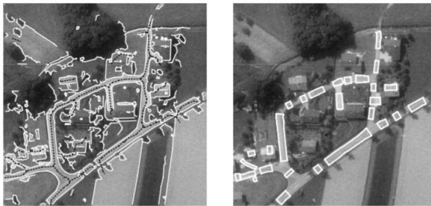
FIGURE 4.3: On the left, input data for the fusion. On the right, hypotheses for road segments. (Preprint [70])
