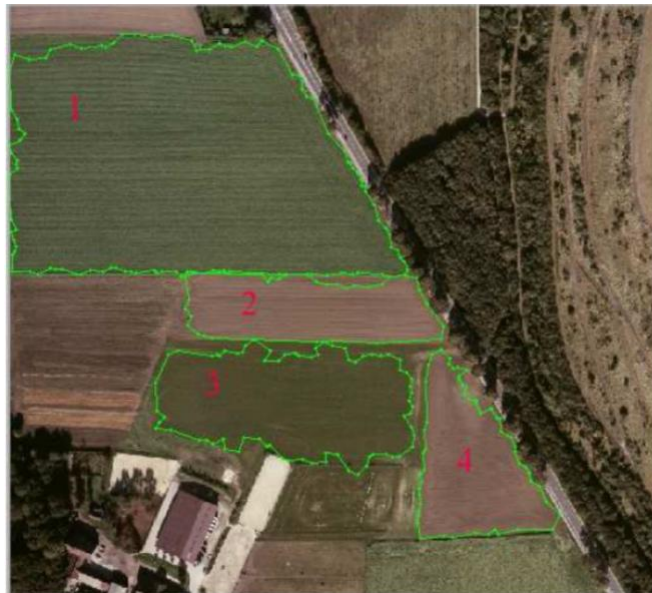
FIGURE 3.8: Color orthophotomap with the results of some fields obtained by semi-automatic extraction.
