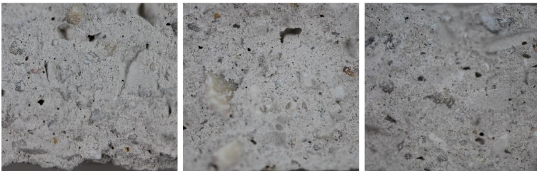
Figure I.12 Stereo microscope images of hardened mortar MD joint sections after 56 days. Magnification 10X.
