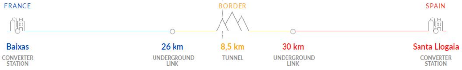
Fig. 1.1: Baixas (France) - Santa Llogaia (Spain) connection (INELFE) [7]
