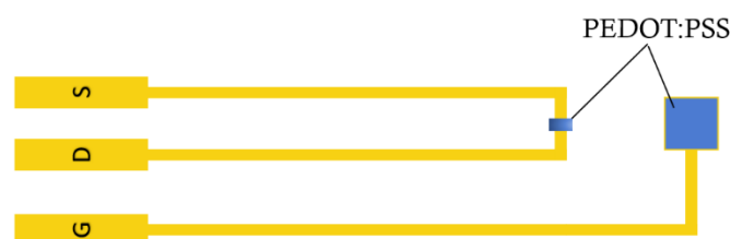
Figure 6.3. Layout of the microfabricated OEET (S: source, D: drain and G: gate).
