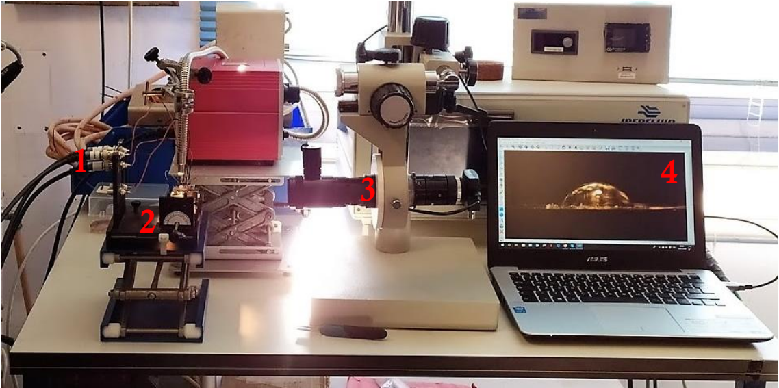
Figure 6.12. Real picture of the setup used for bending measurements. 1: electrical connections. 2: apparatus for the samples bending. 3: optical camera. 4: laptop connected to the camera.
