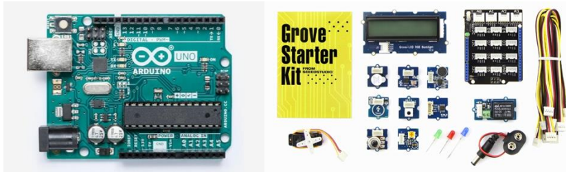
Figure 41. Technological devices used in CREA. Left: Arduino Uno board (image from the Arduino website). Right: Grove starter kit (image from the Grove System website).
