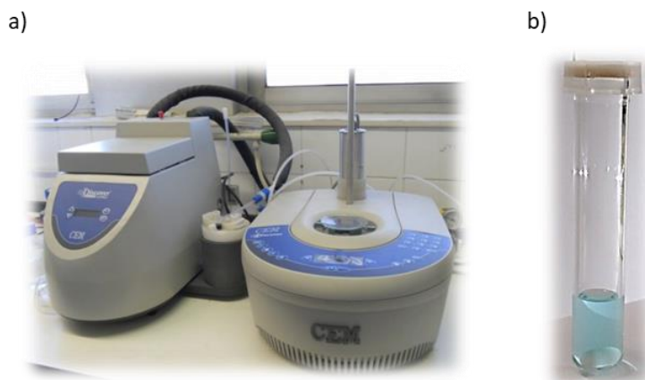
Figure ES-1. a) CEM Discover® microwave instrument used in this thesis work; b) 10 mL glass reaction vessel, sealed with a click septum and equipped with stirring bar.
