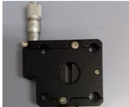
Fig. 4.16: Shows the variable width slit used as a spatial filter.
