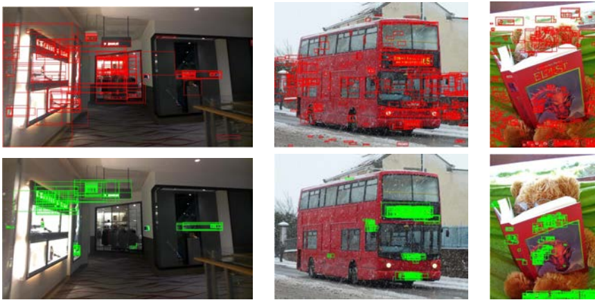
Figure 3.3: Top 500 ranked regions by TextProposals (in red) and by TextProposals with the TextFCN suppression strategy (in green).
