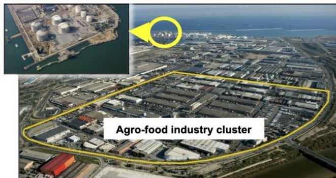
Figure 2.27. Aerial view of the Barcelona LNG terminal (Spain) and neighbouring agro-food industry cluster with refrigeration demand that could utilize the LNG low-temperature exergy.
