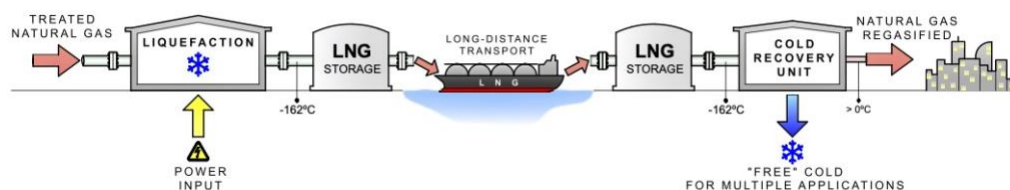
Figure 1.5. A block diagram of the LNG supply chain with the low-temperature energy (cold) opportunity throughout its regasification process [55].
