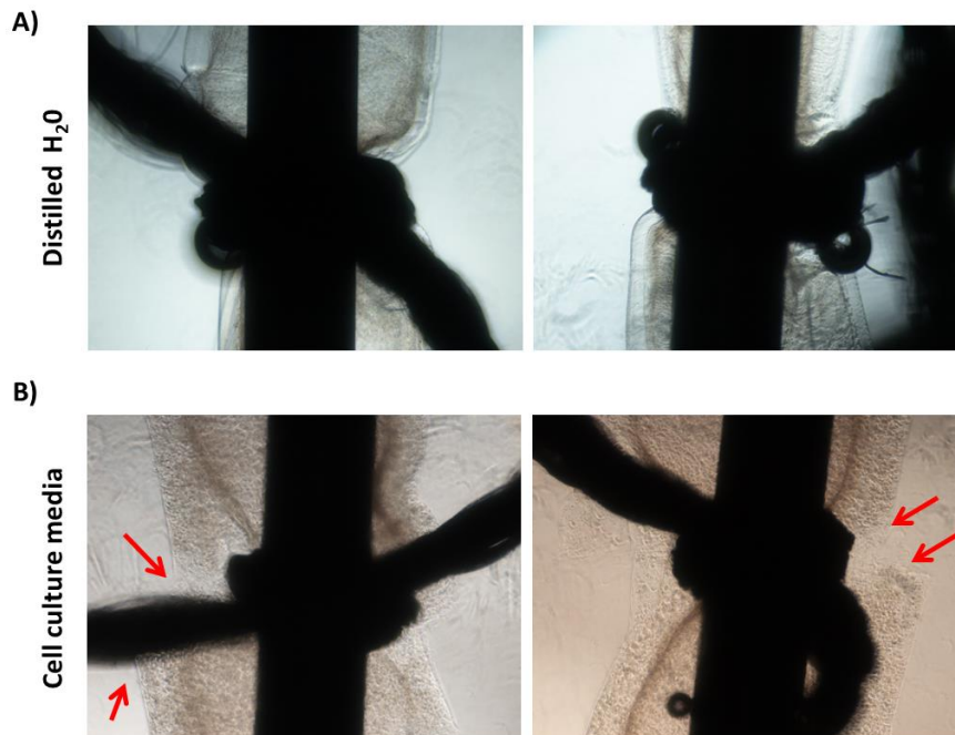
Figure 12. A) Cell-free TEBVs attached with sutures within permeability chamber device in contact with distilled H 2 O. B) Cellular TEBV after 7 days of perfusion in contact with cell culture media. Red arrows show break points of TEBVs.
