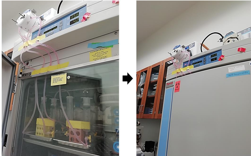
Figure 5. Pictures of the perfusion system with the incubator. Peristaltic pump was placed outside the incubator whereas the rest of the perfusion system was placed inside.
