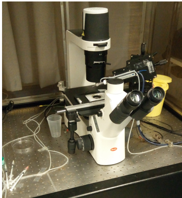
Figure 5.1: Experimental setup for patch-clamp experiment used during the internship in Aarhus to collect the recordings of the membrane potential.
