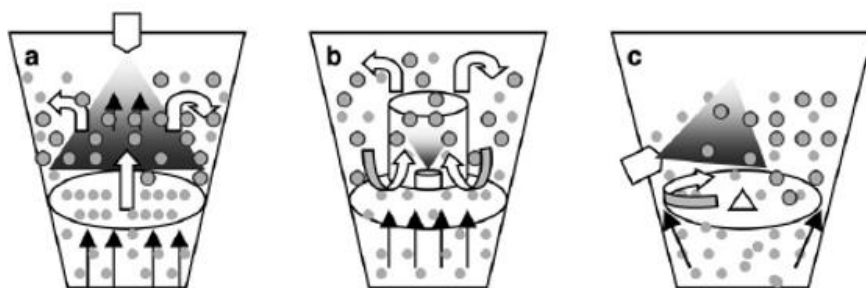
Figure I-7 Schematics of a fluid-bed coater. a) top spray; b) bottom spray; c) tangential spray
