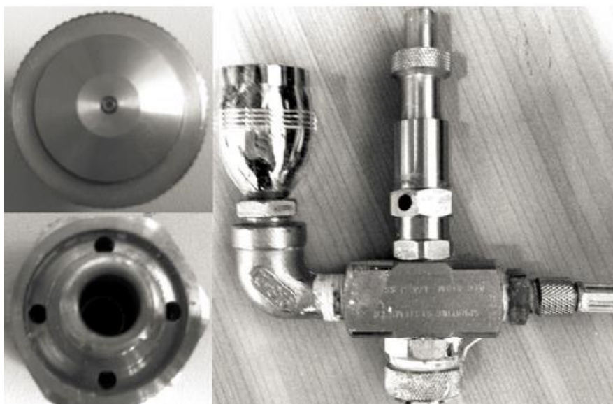
Figure IV-2 Airbrush and nozzle used for IPS technique
