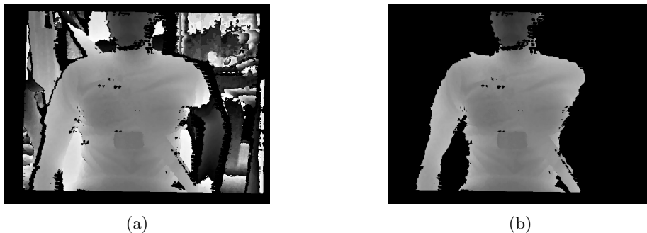
Figure 4.3: a) Point cloud obtained from the Kinect camera, b) cropped point cloud between the distances 500 and 900 mm.
