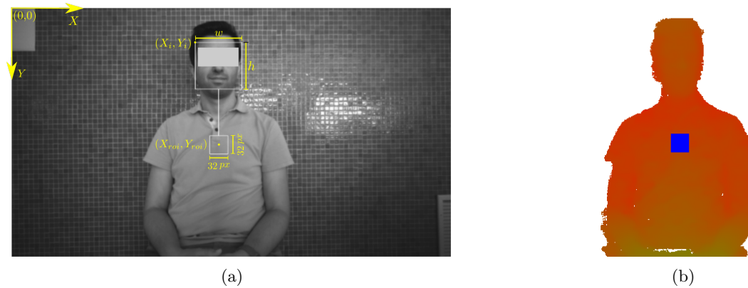
Figure 5.2: a) Depicts the IR frame obtained from the camera, b) depicts the depth point-cloud. In (a) the different metrics used by the method are shown, and referenced to the location of the face. In (b) the computed ROI from the previous metrics is depicted as a blue square. The images correspond to a preliminary study and are not the actual setup. Source: [30] (CC BY 4.0).
