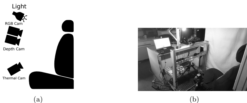
Figure 4.1: a) Depicts the position of the different cameras within the setup, b) depicts the real setup. Figure b) Extracted from: [29], Copyright Elsevier 2019, all rights reserved.
