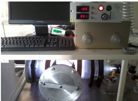
Figure 2. Views of the three plasma polymerization reactor designs assembled in this work. (A) Prototype of a cylinder shaped reactor with parallel plate electrodes and a volume of 20L. (B) Similar design with a reactor volume of 1L. (C) Prototypes of T-shaped reactor with outer ring electrodes, showed left is our first prototype used for all the experimental data presented in this work, and showed right is our second prototype, assembled to be used in related research. (D) A monomer polymerization test with white plasma glow discharge, with view from the side port of the chamber (D, left), and view of scaffold samples placed on the sample holder position (D, right).
