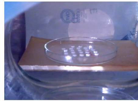
Figure 2. Views of the three plasma polymerization reactor designs assembled in this work. (A) Prototype of a cylinder shaped reactor with parallel plate electrodes and a volume of 20L. (B) Similar design with a reactor volume of 1L. (C) Prototypes of T-shaped reactor with outer ring electrodes, showed left is our first prototype used for all the experimental data presented in this work, and showed right is our second prototype, assembled to be used in related research. (D) A monomer polymerization test with white plasma glow discharge, with view from the side port of the chamber (D, left), and view of scaffold samples placed on the sample holder position (D, right).
