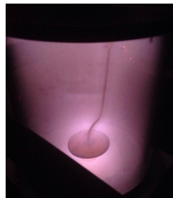
Figure 5. Pictures of first cylindrical chamber plasma reactor prototype. All pictures show the cylindrical chamber (20L) with inner plate electrodes. (A) Whole installation with pump, rf source, matchin unit, monomer inlet and cold trap visible. (B) and (C) show a glow discharge with air plasma with bad electrical grounding, and (D) with a better grounding.
