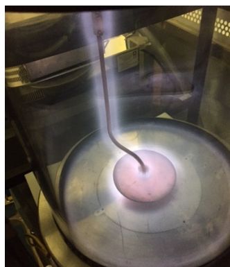
Figure 5. Pictures of first cylindrical chamber plasma reactor prototype. All pictures show the cylindrical chamber (20L) with inner plate electrodes. (A) Whole installation with pump, rf source, matchin unit, monomer inlet and cold trap visible. (B) and (C) show a glow discharge with air plasma with bad electrical grounding, and (D) with a better grounding.
