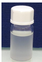
Figure S3. Dispersion of undoped colloidal nanocrystals in apolar solvent (n-hexane).
