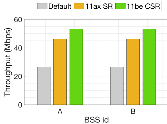
Figure 5.4: Further SR gains provided by CSR in comparison to default carrier sensing and OBSS/PD-based SR.
